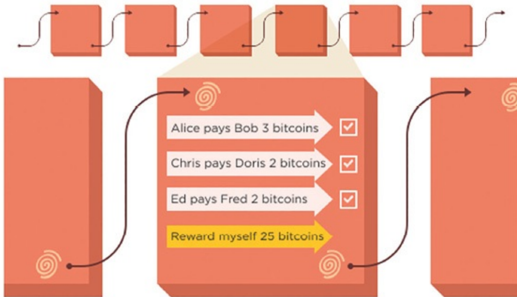
A block chain 96 where each block includes the hash of the previous block, rather than a sequential block number.
